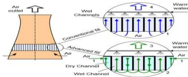
in conventional cooling tower water will pass in all the channel with ambient air. So in this cooling tower operated by sensible heating such as in a tube to air Heat exchanger, they do not use principal of evaporation . but in the advanced cooling tower water and ambient air will pass in separate channel.
