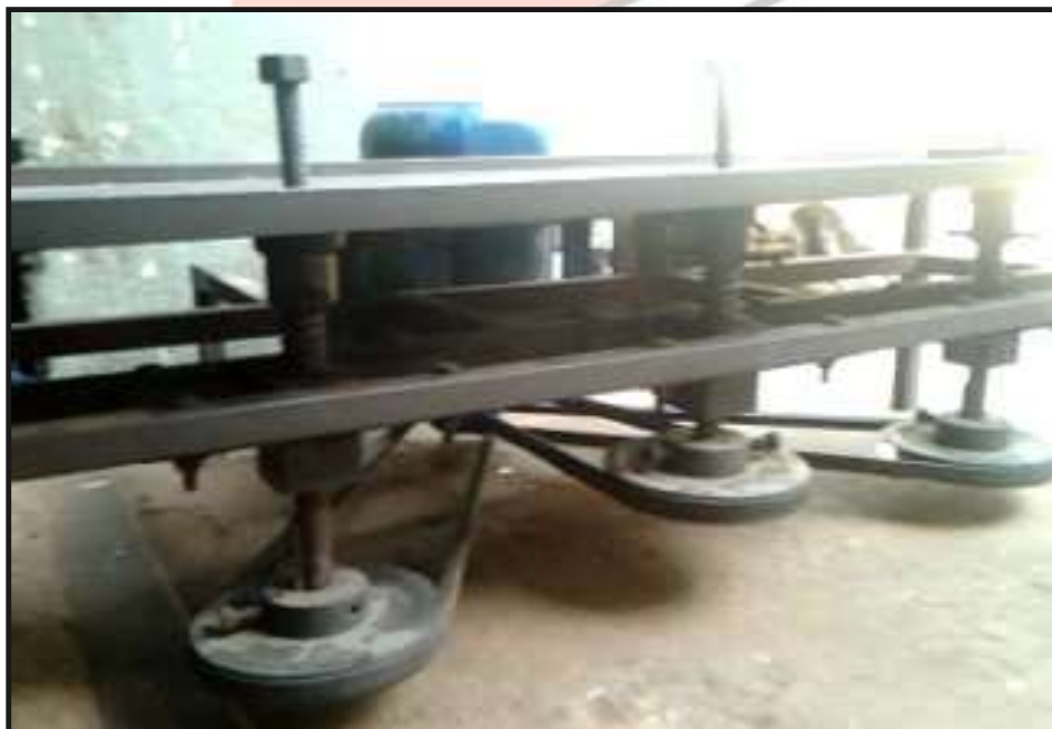
Fig 5. Manufactured Automated Nut Fastening Machine
