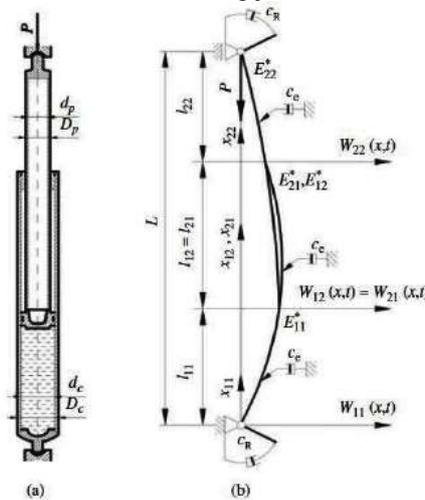
Fig.6. Model Diagram (a) and beam model (b) of a hydraulic cylinder with damping. [15]
