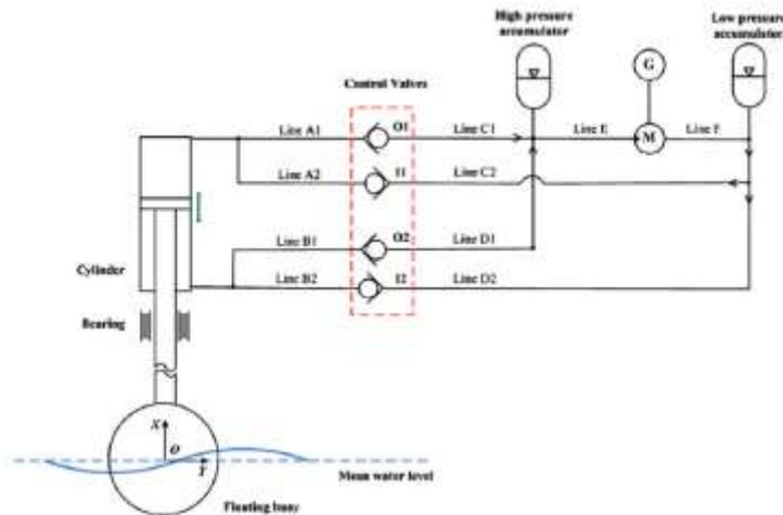
Fig.4. Sketch of wave energy converter consisting of a heaving sphere connected to the hydraulic power take-off [12]
