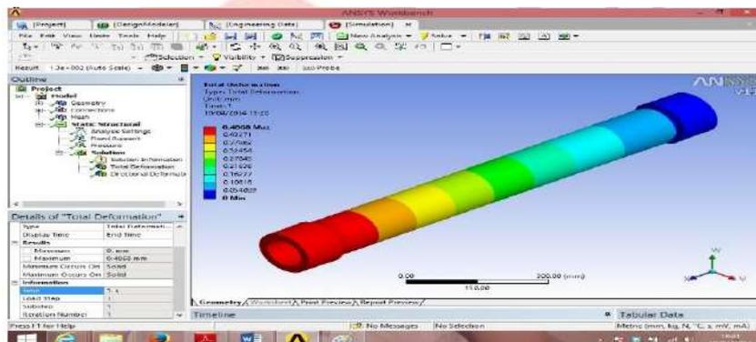
Fig.9. Total deformation of hydraulic cylinder
