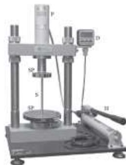
Fig.3 Experimental setup of the press and the cylindrical sample [11]
