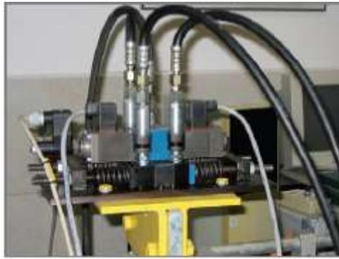
Fig.2 Proportional distributor placed in special holder and bilaterally supported with springs, during testing [7]
