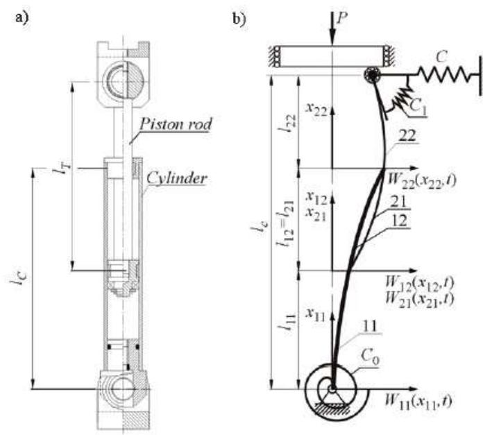
Fig.1 Diagram of the considered hydraulic cylinder:
