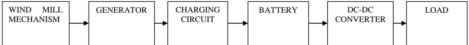
Fig 1. Block Diagram of Regenedyne Wind Power Generation
