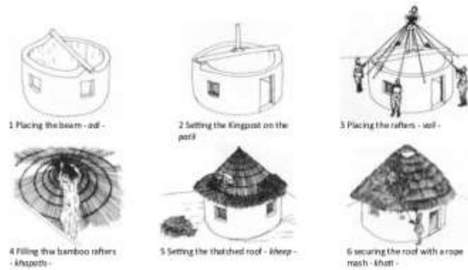
Figure 6: Stages of roof construction.
