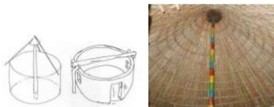
Figure 8: Structural variant for the roof- supported by a central pillar.
