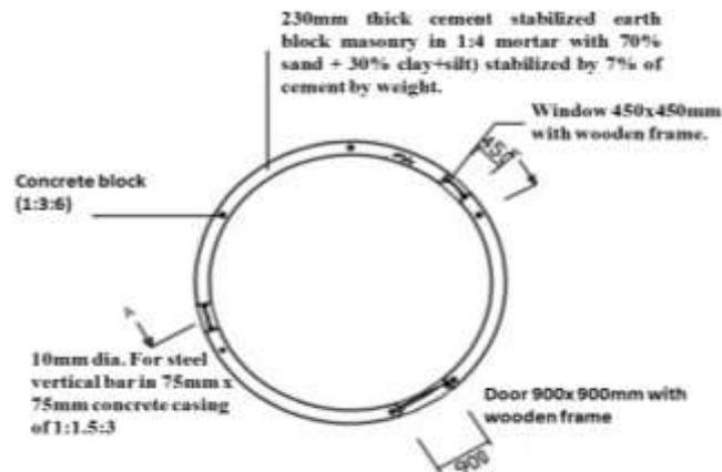
Figure 13: typical plan Stabilized compressed earthen block Bhunga.
