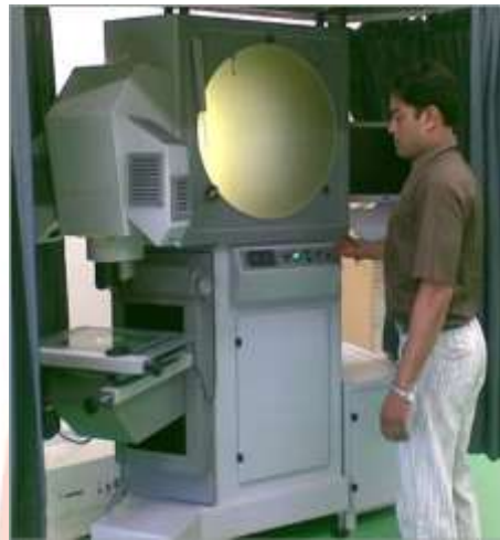
Fig.3. Optical Profile Projector used for finding the depth of penetration
