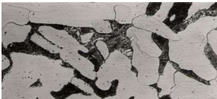
Fig.12: Microstructure of Mild Steel (~0.16 wt% C) showing light-coloured ferrite grains and dark-appearing pearlite regions (Magnification: 500X; Volume fraction of pearlite is estimated to be around 20%)
