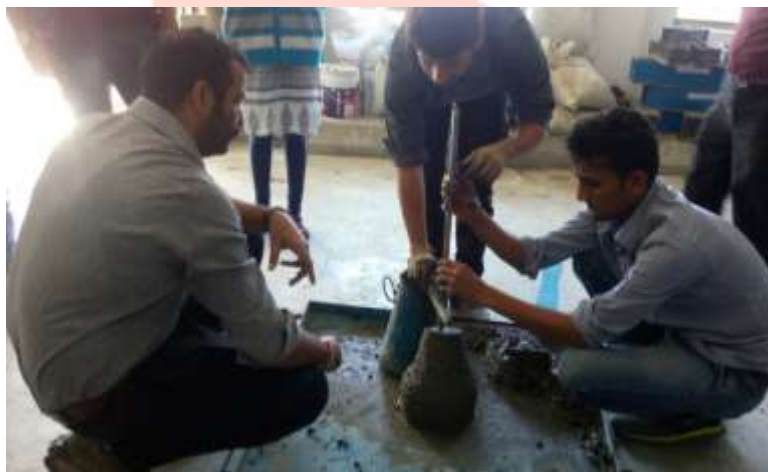
Fig. – 1 Slump Test
