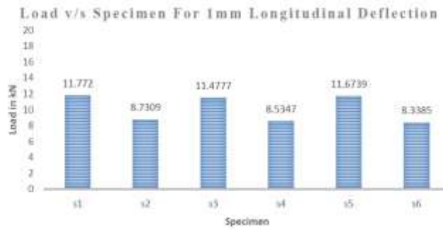
Fig 6 Value of Load Corresponding to 1mm Longitudinal Deflection
