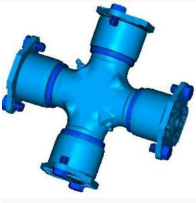
Figure 4: 1710 Series UJ design, [6]
