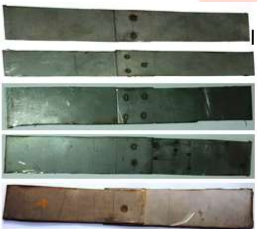
Fig. 2 spot welded specimen before testing
