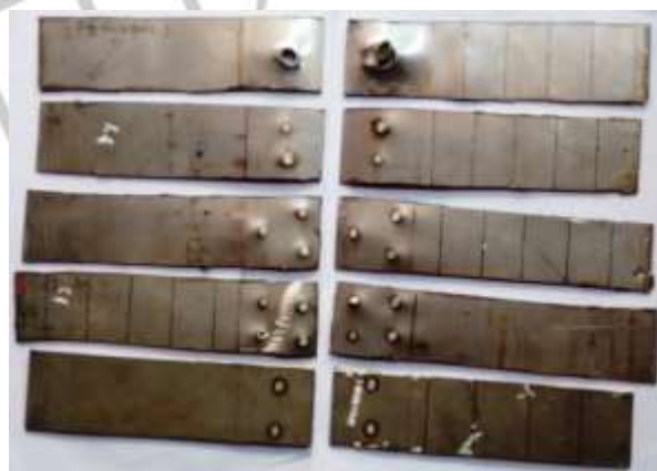
Fig. 3 spot welded specimen after testing
