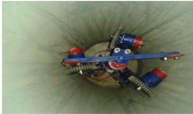
Figure.5.6 working model of pipe crawling machine
