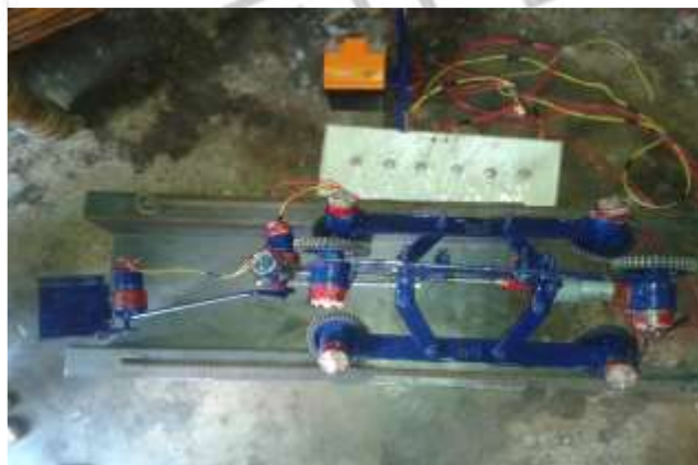
Figure.5.5 working model of open channel drainage cleaning machine
