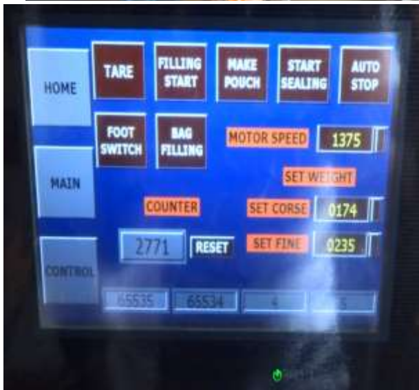
(Fig. 27) Touch Screen for Control the Machine
