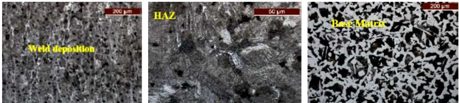
Fig. 2.4: Microstructures of one of the shaft showing transition from weld to HAZ to matrix
