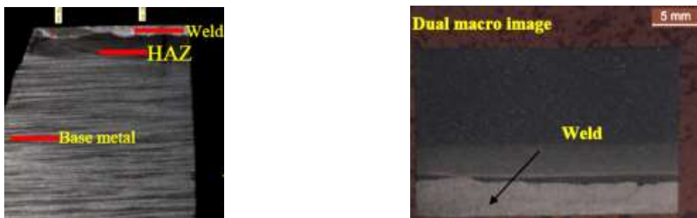
Fig. 2.2: Mounted micro samples of shafts showing distinct regions.
