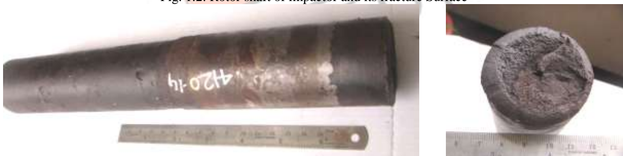
Fig. 1.3: Squeeze Roll shaft and its fracture Surface
