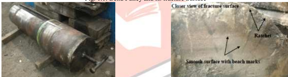
Fig. 1.2: Rotor shaft of impactor and its fracture Surface
