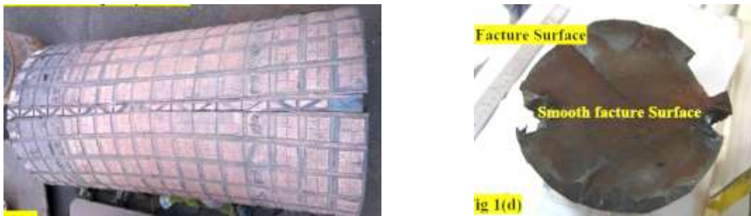
Fig.1.5: Pulley shaft and its fracture Surface
