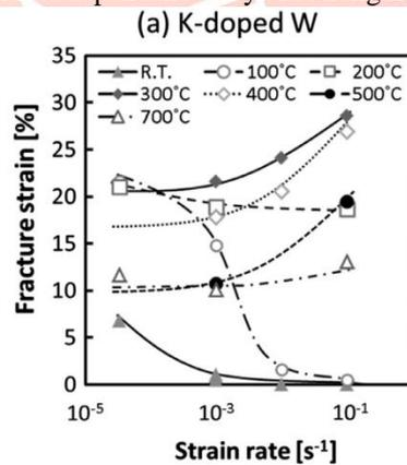
Figure 9-Strain rate dependence of fracture strength (K-doped tungsten)
