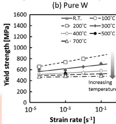
Figure 8-Strain rate dependence of yield strength (pure tungsten)
