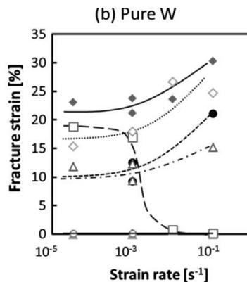
Figure 10-Strain rate dependence of fracture strength (pure tungsten)
