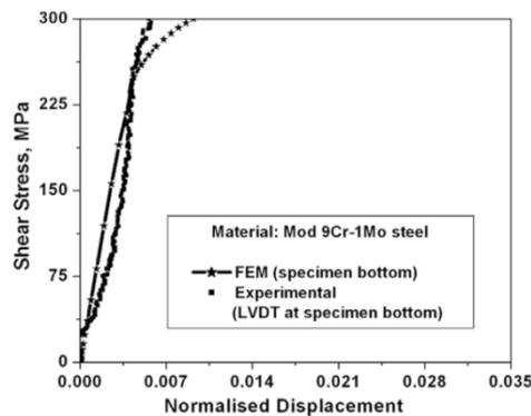
Figure 13-Comparison of FEM results with experimental load –deformation curve
