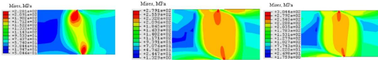
Figure 12-Von Mises stress contour profiles before yield, at yield and after yield
