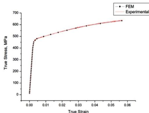
Figure 14- Comparison for true stress- true strain curves
