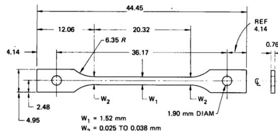
Figure 1- (a) Miniature SS-1 sheet tensile specimen
