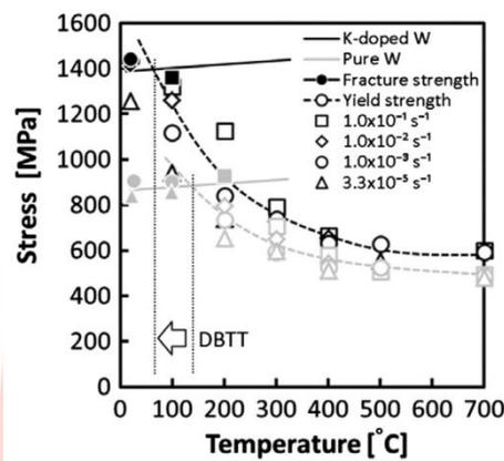
Figure 5- Temperature dependence of UTS of Pure W and K-doped W
