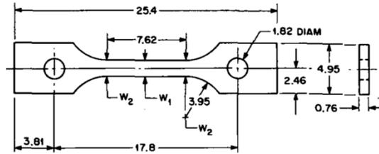
(c) Miniature SS-3 sheet tensile specimen
