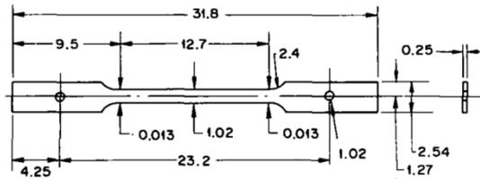
(b) Miniature SS-2 sheet tensile specimen
