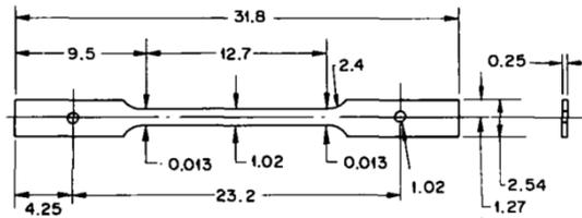
(b) Miniature SS-2 sheet tensile specimen
