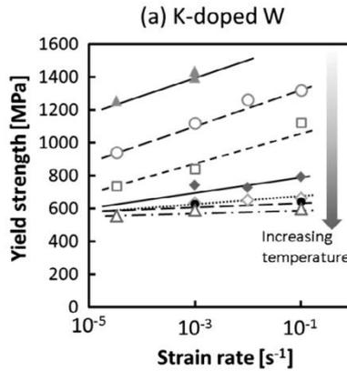
Figure 7-Strain rate dependence of yield strength (K-doped tungsten)
