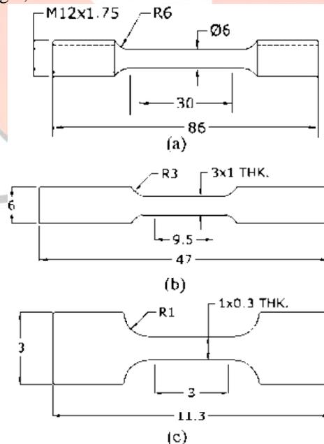
Figure 3-Dimensional details of tensile test specimens
