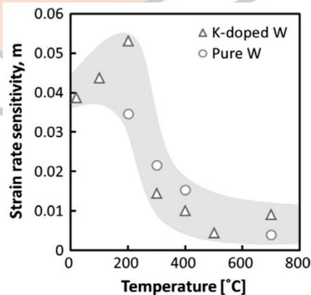
Figure 6-Temperature dependence of strain rate sensitivity
