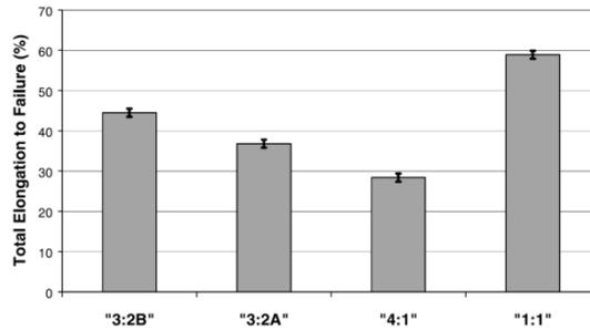
Figure 2-Total elongations to failure as a function of specimen geometry
