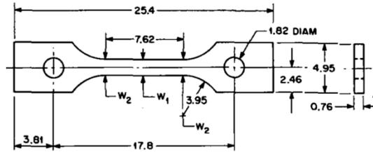
(c) Miniature SS-3 sheet tensile specimen
