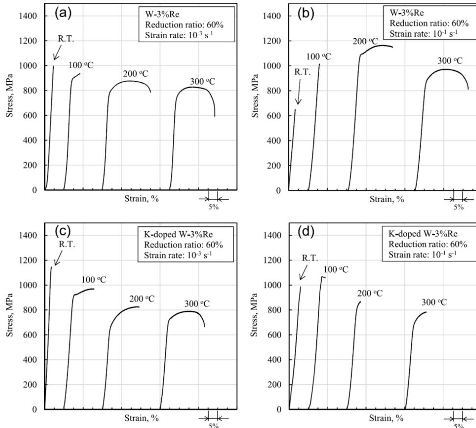
Figure 11- Engineering stress–strain curves obtained by tensile test of W-3%Re and K-doped W-3%Re.
