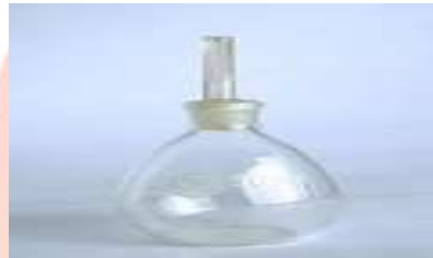
Figure No.1 Specific gravity bottle for cement Result obtained G=3.1
