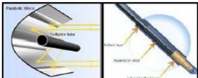
□ The reflector can be made from Glass mirror and aluminum foil .one disadvantage of a parabolic
