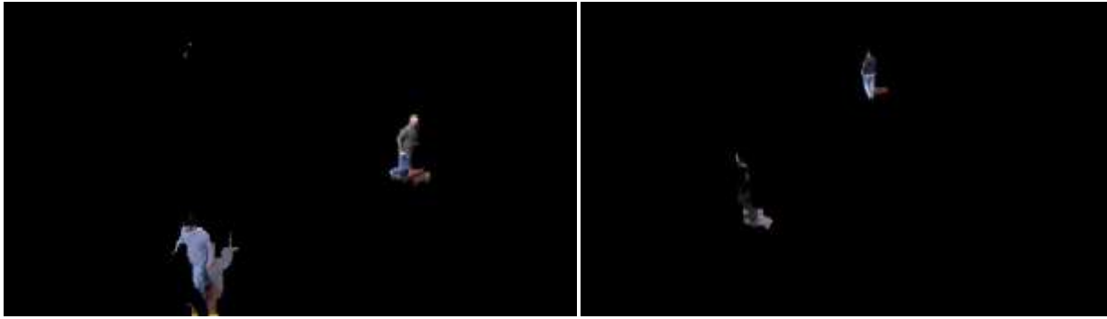
Fig.3: Representing Background Subtracted from the Frame
