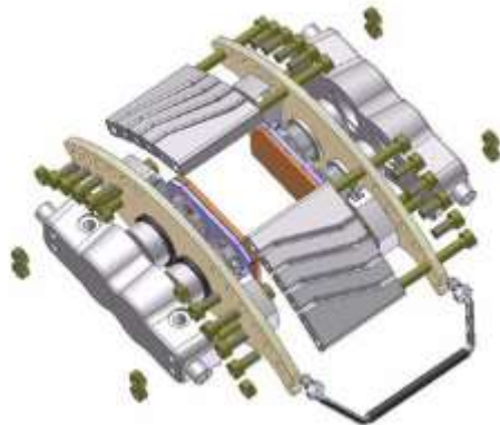
Figure 4-8: Exploded view of the modular caliper assembly
