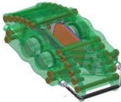
Figure 4-5: Internal structure of modular brake caliper assembly
