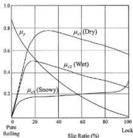
Fig. 3 – Relation between longitudinal, lateral friction coefficients and slip ratio [3]
