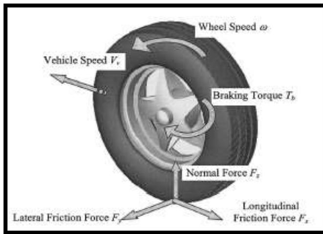
**Figure: 2. Modelling wheel for slippage mechanism (Courtesy: [5])**
