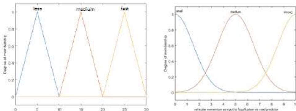
**Figure 5: Membership functions for vehicular momentum and speed for fuzzifier**
