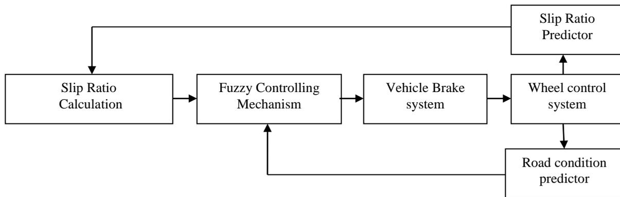
**Fig. 4 – ABS Fuzzy Control System for Vehicles**
