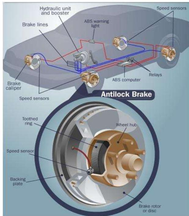
**Figure: 1. General ABS System with components**
