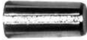
Figure 7. Roller defect at 0°
