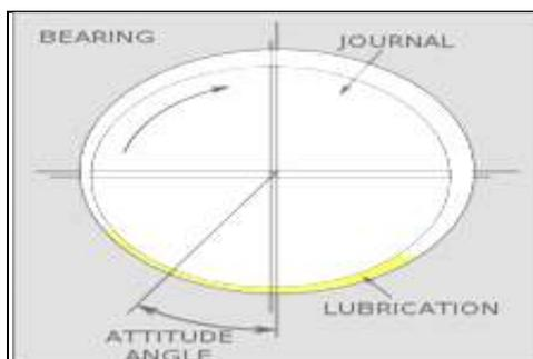
**Figure: Fluid Lubrication**
