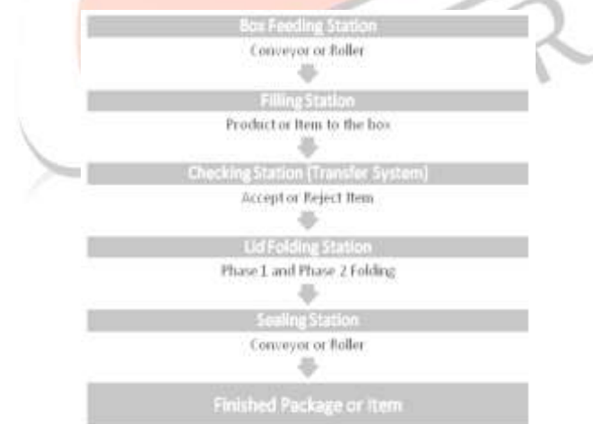
Fig 1.Diagrammatic structure of automated system
