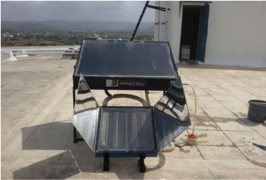
Fig 1. Experimental setup of advanced solar distillation system.
