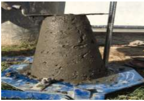
Fig 1.16 Subsidence of Slump Test
