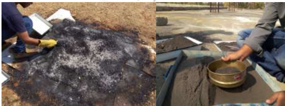
Fig 1.6 collecting saw dust ash Fig 1.7 Sieving saw dust ash with IS 90 microns
