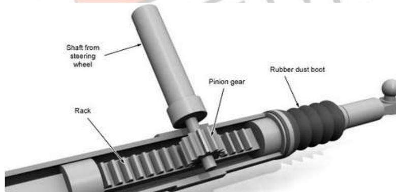
**Fig 7: Depiction of Rack and Pinion for steering**
