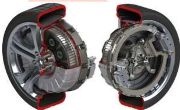
**Fig 2: In-wheel motor**
