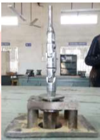
Figure 5. View of square hole drilling machine and special tool
