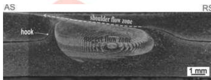
Fig.10. Cross sectional view of an AZ31B weld made using \omega = 1,000 rpm and v = 112 mm/min displaying a large hook
