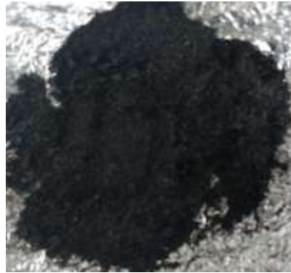
Fig. 7: Carbon made from Sugarcane Bagasse
