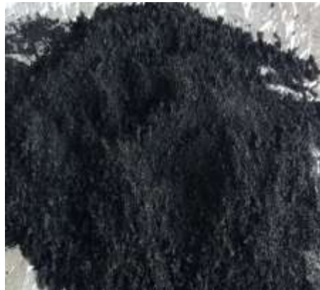
Fig. 4: Carbon made from Rice Husk
