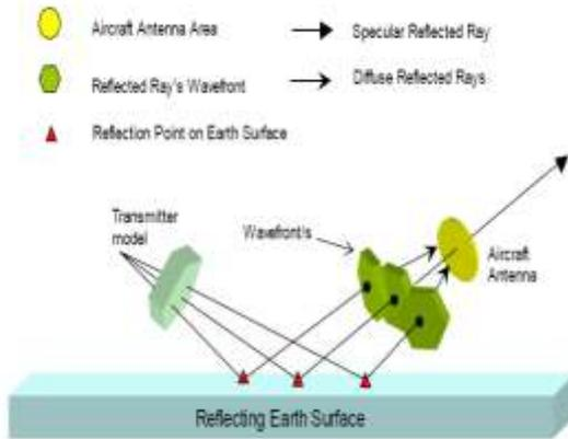
Fig.3. ray tracing transmitting model
