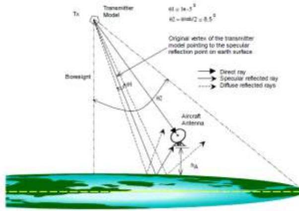
Fig.5 Satellite to aircraft ray tracing model
