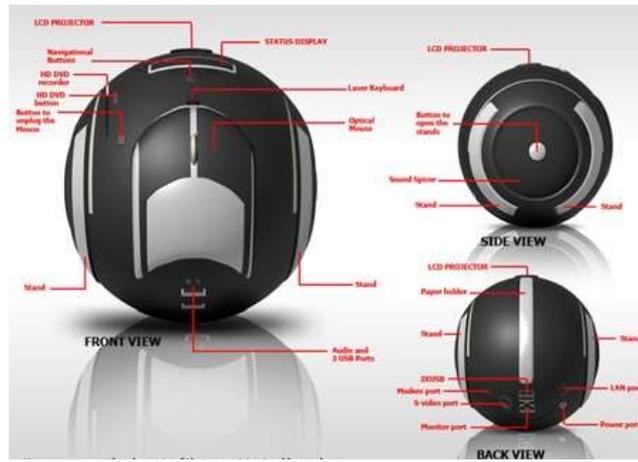
**Fig. 2. Element of E-ball computer**
