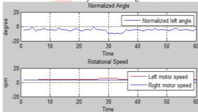
Figure 7: Graph of speed variation in left and right wheel [11]
