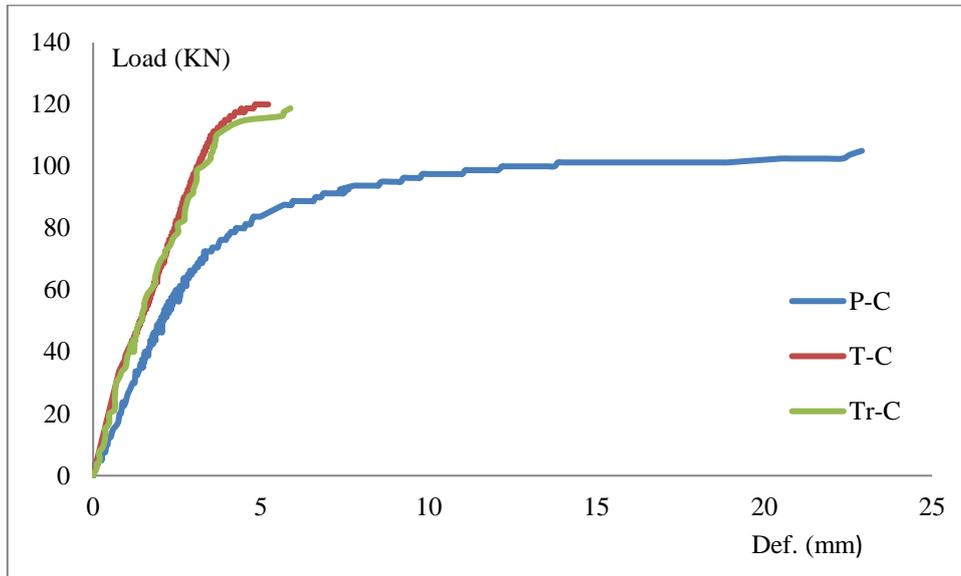
Figure (16) comparison between the three CHTFB at Ultimate load for each tested beam
