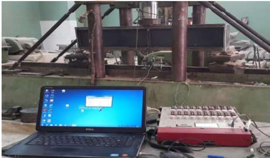
Figure (4) testing system showing LVDT, Load cell and data logger
