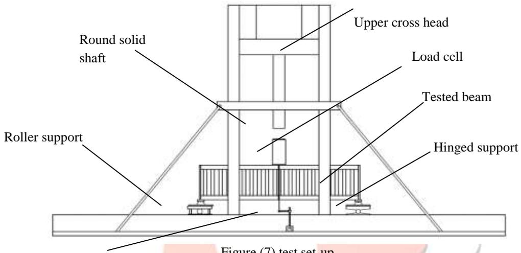
Figure (7) test set-up
