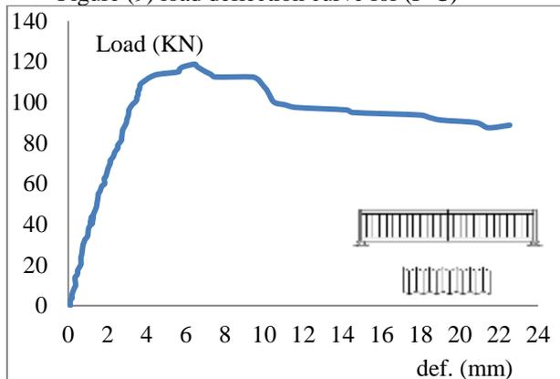
Figure (11) Load-deflection curve for (Tr-C)
