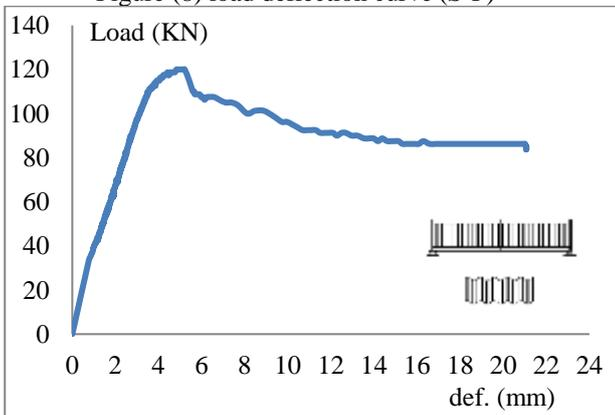
Figure (10) load-deflection curve for (T-C)
