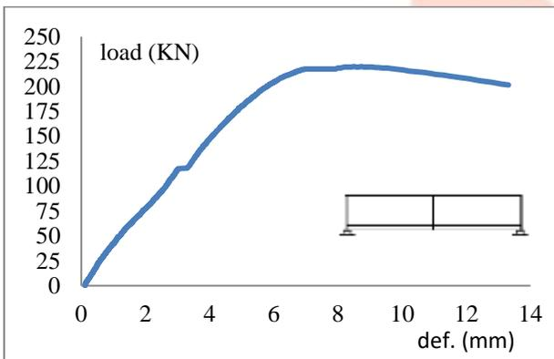
Figure (8) load deflection curve (S-P)
