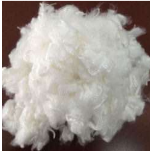
Fig. 1. Loose 6mm polyester Recron Fiber
