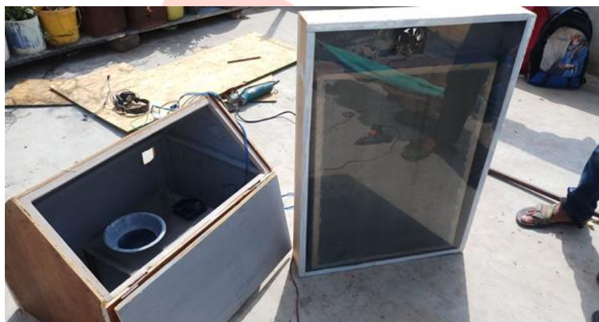
Fig.1 Final Assembly of Solar Green House Drying
