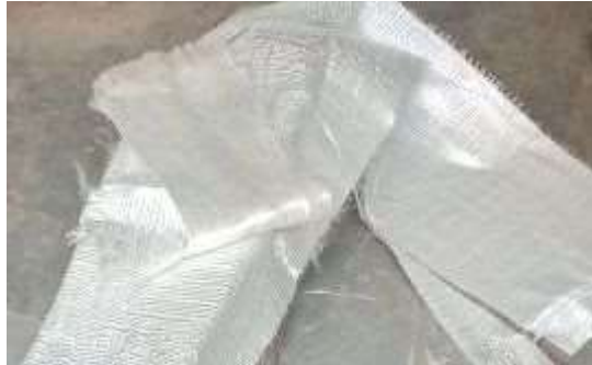
Fig: (a) (GFRP) Laminate of thickness 1.2 mm for strengthening of beams
