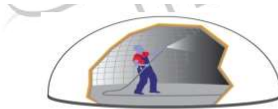
Figure.5 - Spraying of Shotcrete
