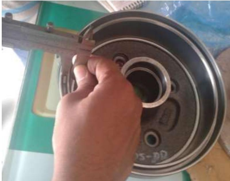
Figure 2.1 New Drum brake for Ra value
