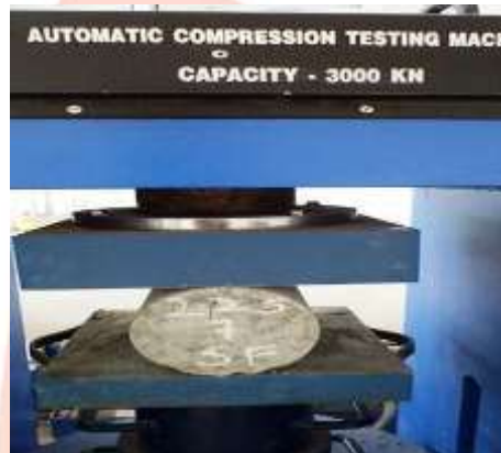
Figure No. 2.6.2. Split tensile strength test
