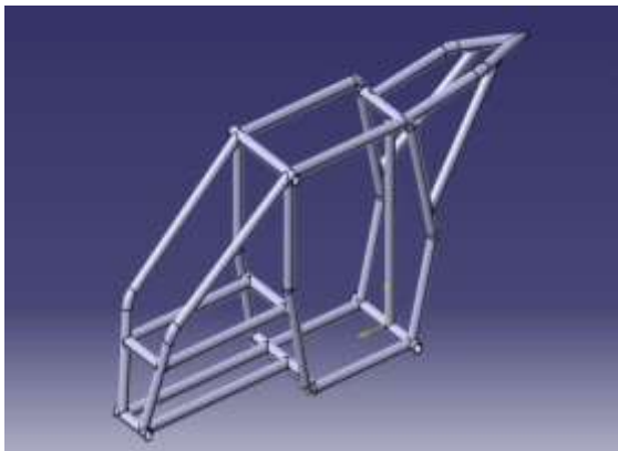
Fig. 1 CATIA model of Chassis
