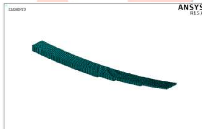
Fig 4.2 Meshed Multi Leaf Spring Model
