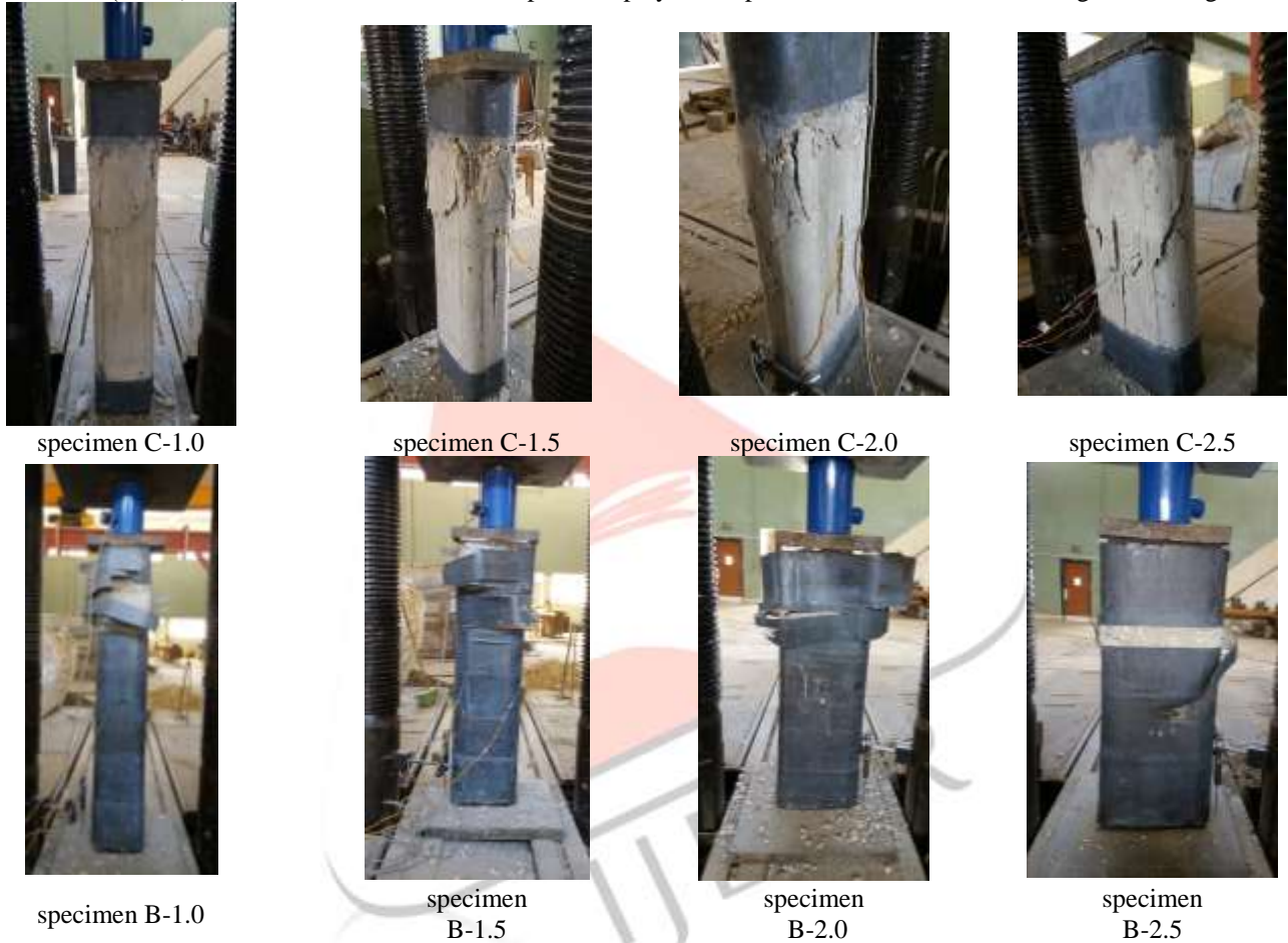
Figure 3: Failure modes for the tested columns.
