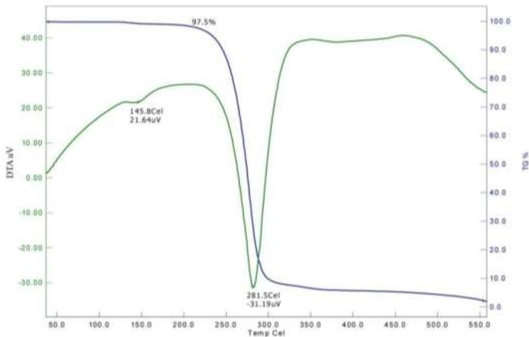
Fig. 3. TGA/DTA spectrum of LVCC crystal doped with zinc chloride
