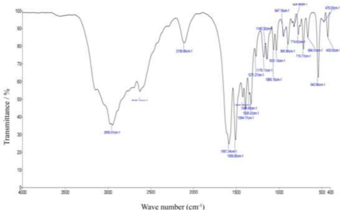
**Fig.2**FTIR spectrum of LVCC crystal doped with zinc chloride
