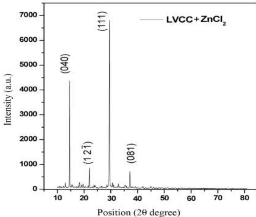
**Fig.1**The powder XRD pattern of the grown LVCC crystal doped with zinc chloride
