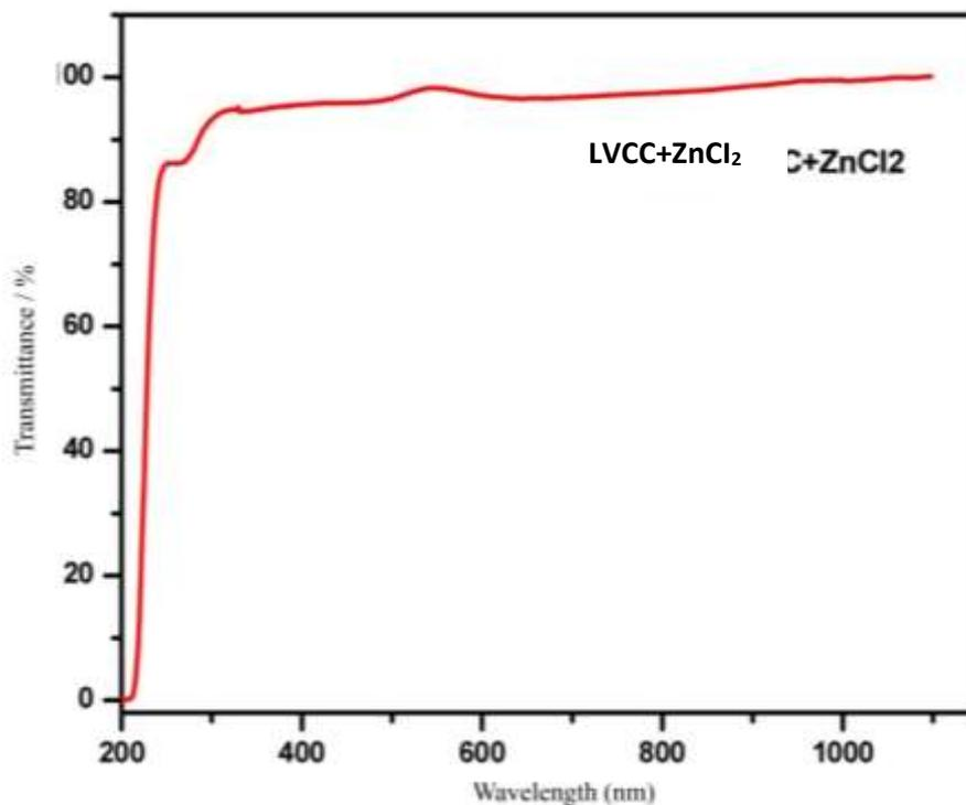
Fig. 4 The optical transmission spectrum of the grown LVCC crystal doped with zinc chloride
