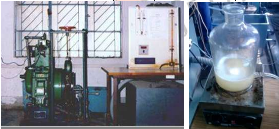
Figure.2 Single cylinder diesel engine test rig with magnetic stirrer setup
