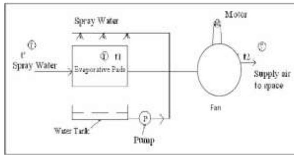
**Figure 1.1 Basic process of evaporative cooling**
