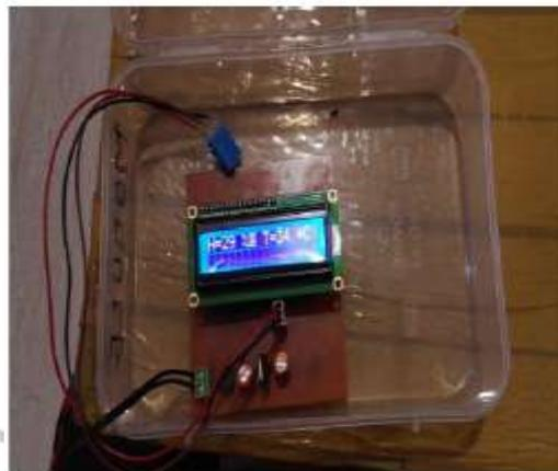
**Figure3.4 Temperature and Humidity measuring device**
