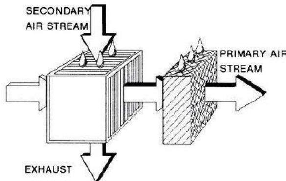
**Figure 1.3 Indirect- Direct (Two-Stage) Evaporative Cooler Airflow Paths**
