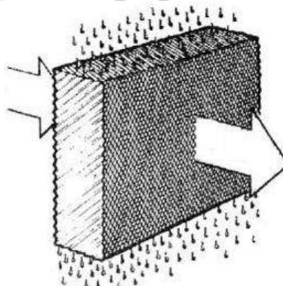
**Figure 1.2 Direct (single-stage) Evaporative Cooler Airflow Path**
