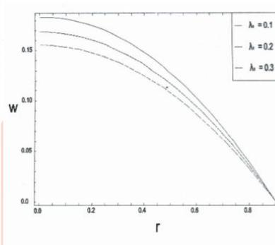
Fig 3: Velocity profiles for different Jeffrey Parameter  $\lambda_1$  in the second stenotic region  $B_1 - \frac{L_2}{2} \leq z \leq B_1$
