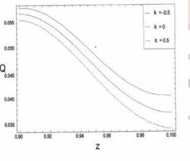
Fig 6: Volumetric Flux for different k in the third stenotic region  $B_1 \leq z \leq B_1 + \frac{L_2}{2}$
