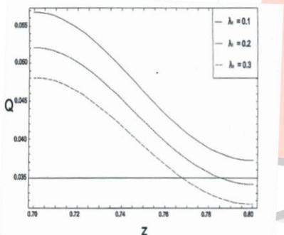
Fig 5: Volumetric Flux for different Jeffrey parameter  $\lambda_1$  in the second stenotic region  $B_1 - \frac{L_2}{2} \leq z \leq B_1$
