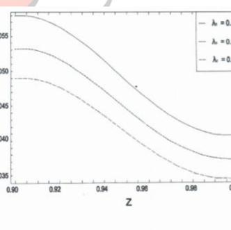
Fig 7: The Volumetric Flux for different Jeffrey parameter  $\lambda_1$  in the third stenotic region  $B_1 \leq z \leq B_1 + \frac{L_2}{2}$
