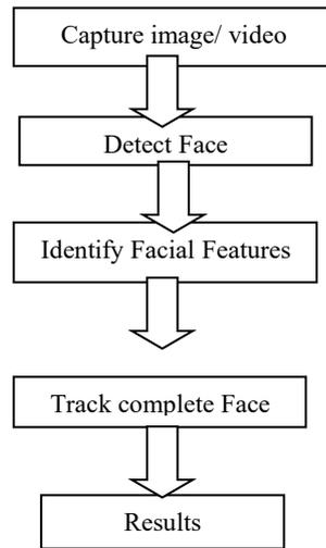
Figure. 2: KLT Algorithm Flowchart
