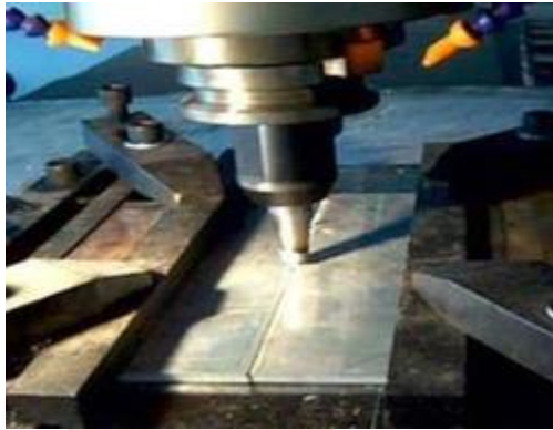
Fig.2. Friction stir weld on aluminium metal alloy
