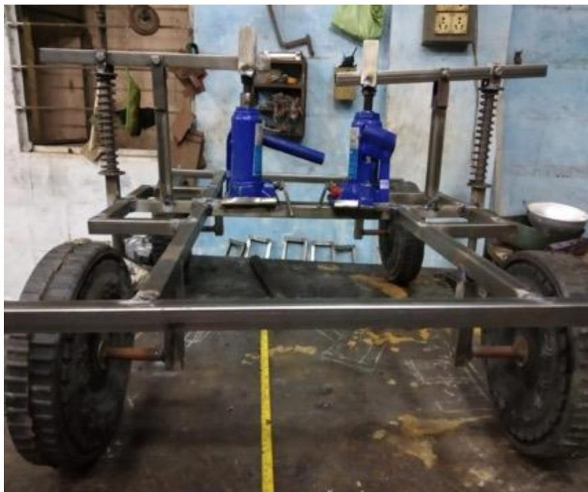
Fig 1.4 Image of the chassis frame fitted with hydraulic jacks.
