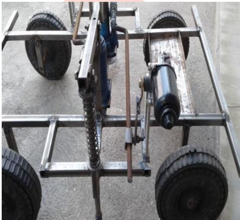
Fig 1.3 Image of arrangement of components on the chassis frame.
