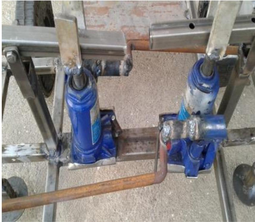
Fig 1.2 Image of two hydraulic jacks fitted on the frame.
