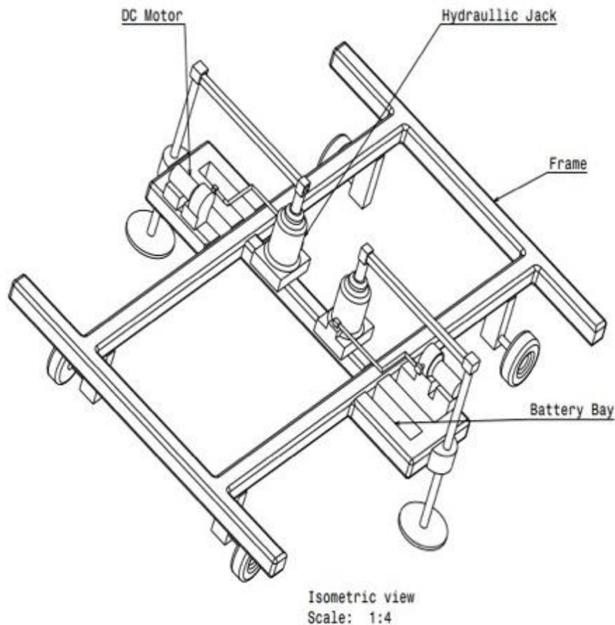
Fig 1.1 Schematic representation of Self-Jacking mechanism in four wheelers.
