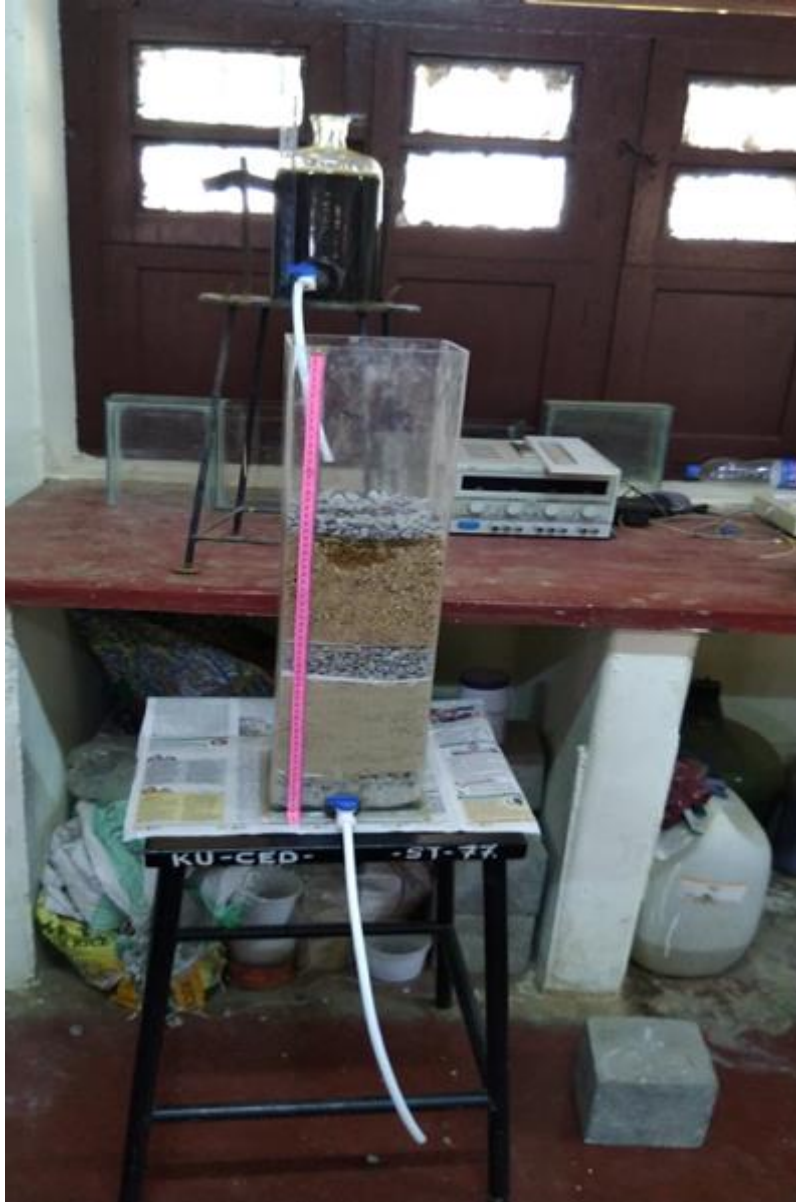
Fig 2: Photographic View of Stratified Soil Bed
