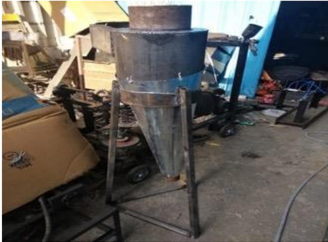
**Fig.8 1D3D Cyclone separator**
